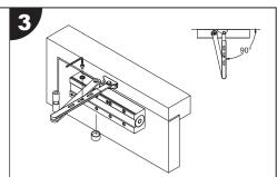
Connect the armset ensuring the pre-loading requirement has been completed.
