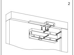
Using the templates provided, fix the mechanism to the door as well as the armset and parallel arm bracket.
