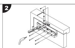
Using the templates provided, fix the mechanism to the door as well as the armset and any necessary brackets.
